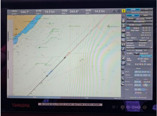
AIS data displayed on the ECDIS, including available information such as object type and reported distance, is utilised.
